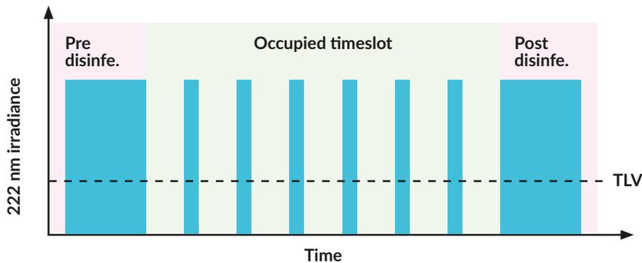
If movement in the room is detected during the pre or post disinfection cycle, the unit will start its duty cycle again, and will resume its pre or post disinfection cycle after no more movement is detected.
