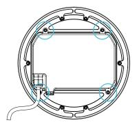
Insert the front plate on the ceiling hole, and apply joint sealant.
