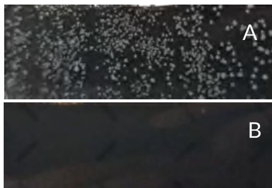
*Figure 7. Mask sample before irradiation (A), Mask sample after a dose of  $10 \text{ mJ/cm}^2$  (B).*
